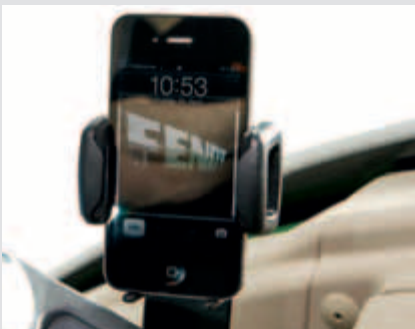
A bracket keeps mobile phones their own fixed spot. The bracket can be adjusted to accommodate various phone models.
