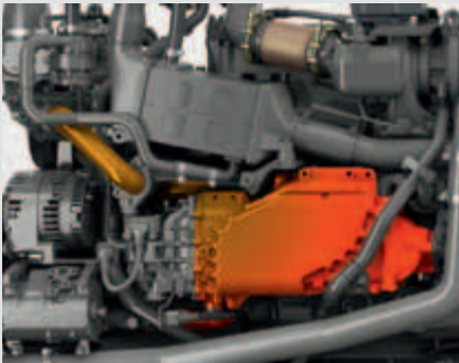
The external exhaust gas recirculation ensures that the nitrogen oxides Nox are already reduced before they reach the exhaust line. That is more economical, because less AdBlue is required in the exhaust line to further reduce the nitrogen oxides.
