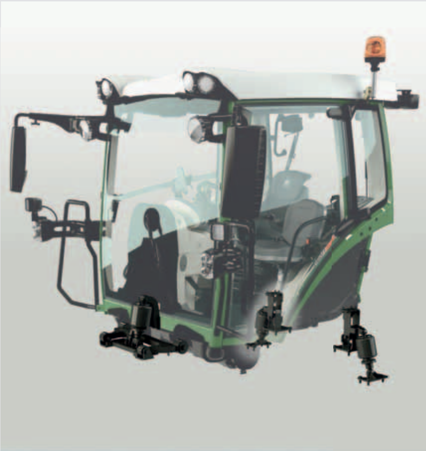
The cab suspension with air spring elements enables a fully vibration-minimised cab. The great difference in height and the long distance between the spring elements of the x5 cab also prevent bouncing and ensure maximum ride comfort.
