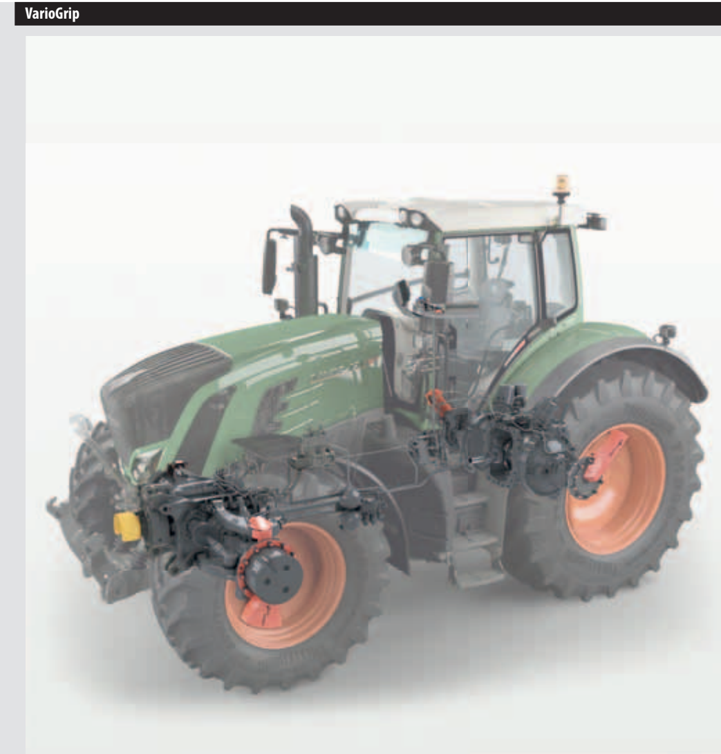
The tyre pressure regulation system allows pressure to be controlled while driving. This is accomplished via the integral rotary union, which is designed to last the lifetime of the tractor. Air is supplied via a modified vehicle compressor as well as the vehicle's own valve equipment. The tyre pressure can be increased by one bar within ten minutes. Reducing pressure by one bar takes only two minutes.
