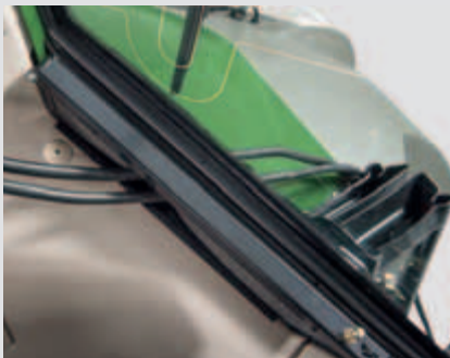
Fendt offers a clever solution for cables that run from the rear of the tractor into the cab. Cables can be guided through the lead-through, no matter what kind of cross section they have. The rear window can be closed, so dust, dirt, water and noise stay outside.
