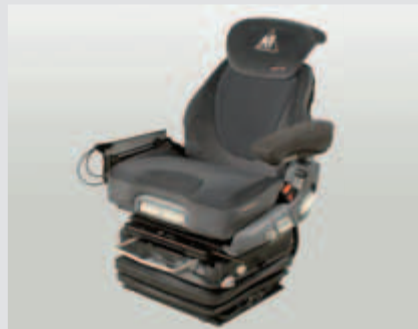
In addition to the features of the super comfort seat, the premium high-tech version of the seat also offers active suspension. This reduces operator fatigue during long periods of work.
