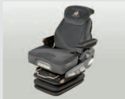
The air-suspended super comfort seat is equipped with heating, a rotary adapter, low frequency suspension, pneumatic lumbar support and easy armrest adjustment. Furthermore, it has climate control and dynamic damping. The compressed air compressor is located outside of the cab, where the noise cannot disturb the operator.
