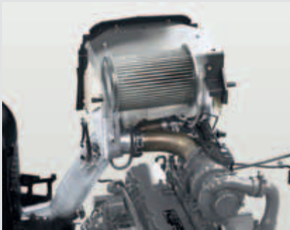
The passive coated soot filter is regenerated while driving and does not need to be actively started. No additional fuel is required for regeneration. The coated soot filters in Fendt tractors are designed for a long life, replacement is not necessary.
