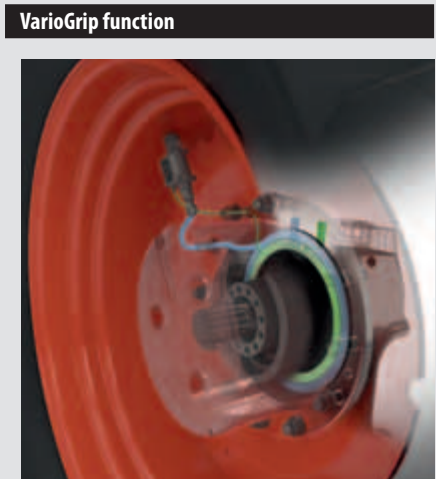
The lines for the VarioGrip tyre pressure regulation system run through a radial rotary union. The air in the tyres is pumped in and out quickly through a control (green) and air line (blue).
