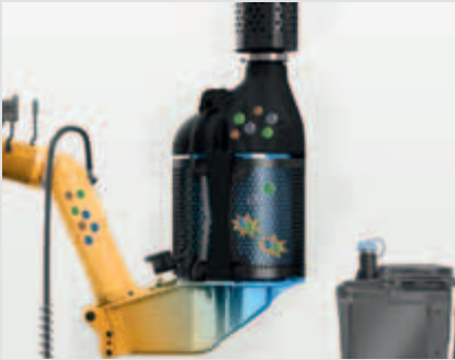
With SCR technology, exhaust is after-treated with AdBlue®, a 32.5 percent solution of urea, which converts nitrous oxides NOx into non-toxic nitrogen and water.
