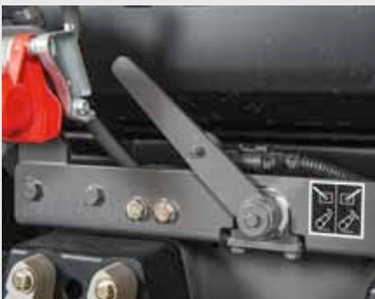
The lower links can be fixed in place through a shut-off cock on the rear linkage, so they cannot move upwards.
