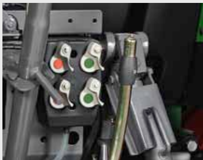
Both the DCUP and CUP couplings permit the hydraulic valves to be coupled under pressure and mounting and removing implements is easy. The self-closing valve flaps offer secure protection against contamination through dirt or water.
