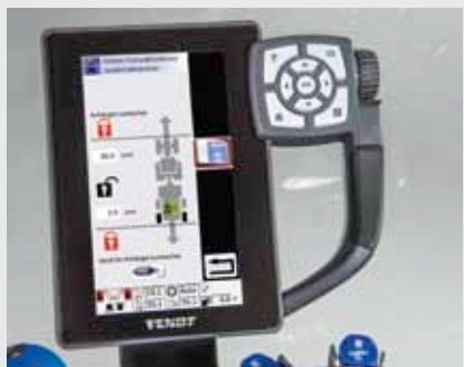
The optional automatic steering axle lock automatically unlocks the steering axle at a predefined speed on trailers with self-steering axles. On straight stretches, the locked self-steering axle ensures stable handling. Operators do not need to lock the self-steering axle manually outside of the preselected speed range and when reversing.
