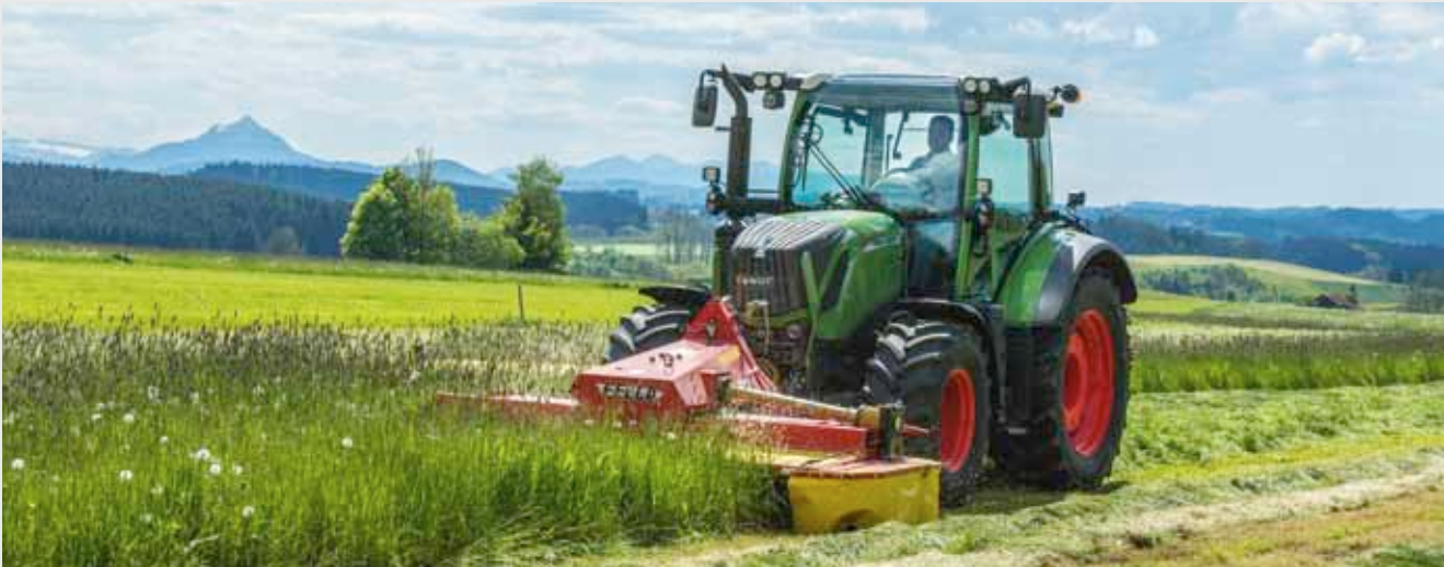
The load relief front linkage control is a special advantage for operations with a front mower in grassland, with front mulching implements, as well as with a snow plough, since the implement adapts to uneven ground very quickly.
