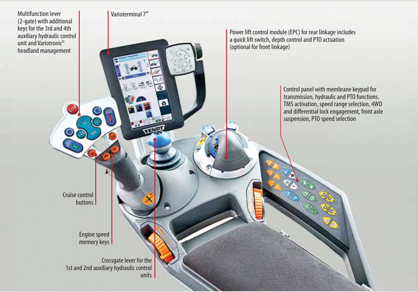
You can operate and monitor all the functions of the Fendt 700 Vario Power in the terminal. Simply touch the corresponding menu item directly on the touchscreen or click a key. With 262,000 colours and a clear resolution of 480 x 800 pixels, all content can be recognised quickly and easily. The display dims automatically at night, without blinding.
