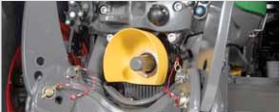
The integrated front PTO delivers 1000 rpm. The direct drive line from the engine to the implement means high efficiency. Another advantage of the foldable lower links is that implements can be attached closer to the tractor and access to the front tyres is better.
