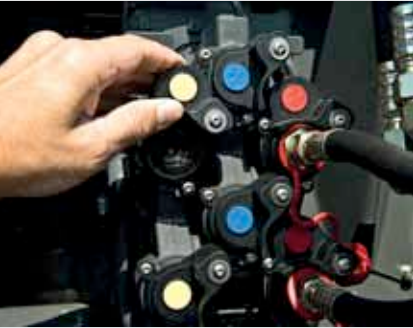
Both the DCUP and CUP couplings permit the hydraulic valves to be coupled under pressure; mounting and removing implements is easy. The self-closing valve flaps offer secure protection against contamination through dirt or water.
