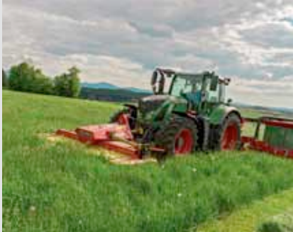
The load relief control for the front linkage is a particular advantage when operating a snow plough or a front mower in grassland operations, since implement guidance can be quickly adjusted to uneven surfaces.
