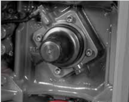
Rear PTO with 540, 540E, 1,000 and 1000E rpm speeds The external PTO actuation at the rear is especially convenient.
