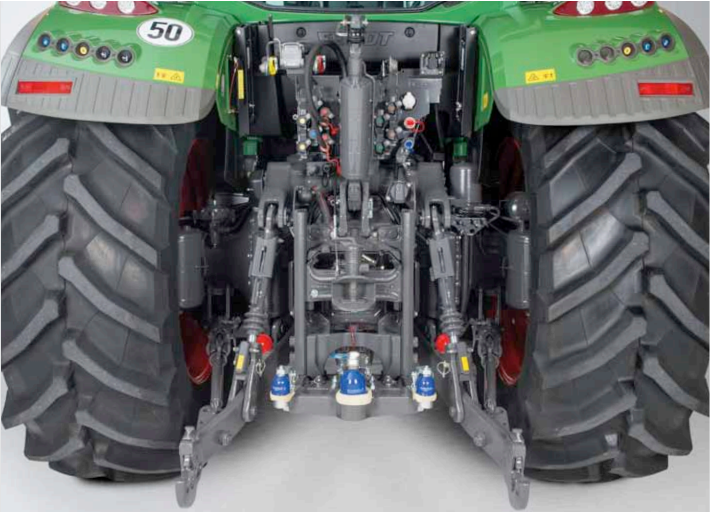
All the interfaces at the rear are arranged functionally and clearly. Signal socket, hydraulic top link, up to five spool valves, unpressurised return, compressed air brake, pressure and control line power beyond, hydraulic trailer brake, 7-pin socket, lower link catch hooks, ABS socket, hitch, rear PTO 540, 540 E, 1000 and 1000E rpm, bottom hitch and steering axle automatic.
