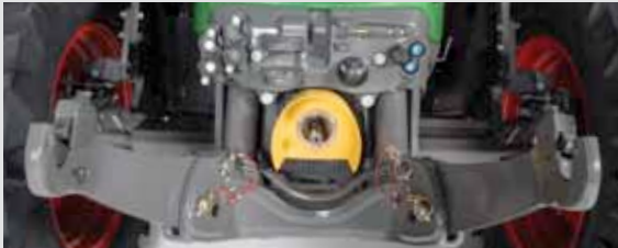
The front linkage is fully integrated in the half-frame and therefore especially stable. The lower links on the front linkage can be folded up diagonally, which provides more clearance for front loader work.
