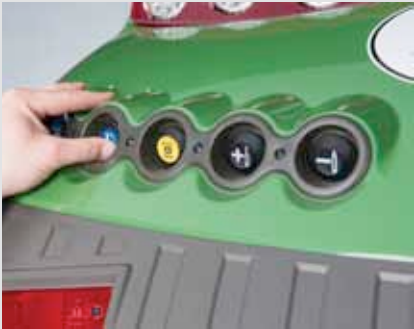
The valves can also be operated externally on the rear mudguard, which makes mounting implements much easier.
