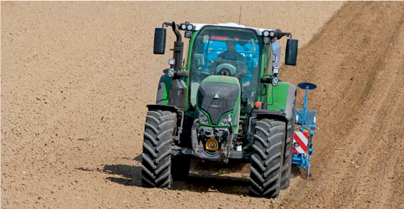
The Fendt 700 Vario offers you the best solutions for your individual requirements in three equipment variants – Power, Profi and ProfiPlus. A number of features and mounting areas are already found in the front alone: top link, up to two double-acting control valves, unpressurised return front, seven-pin socket, front PTO (1000 rpm), EPC front linkage incl. shock load stabilising, lower link catch hooks, foldable lower links, shut-off cock;
