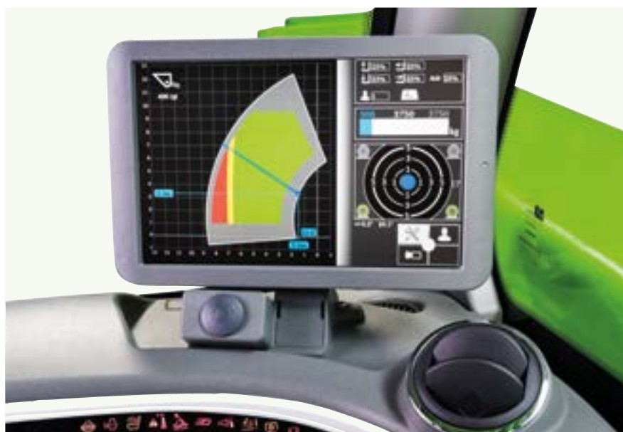
Merlo ASCS (Adaptive Stability Control System) rated capacity limiter
