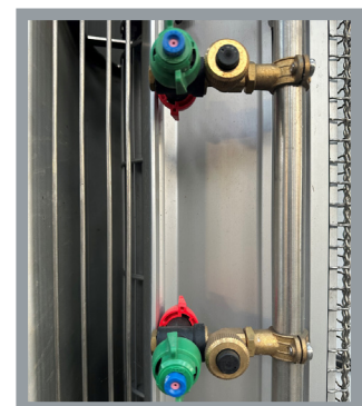
Fan with wet boom
