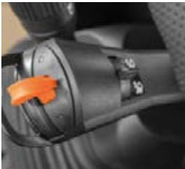
2 programmable lighting modes Use the switch on the reverse lever to quickly toggle between two stored lighting modes, including road and field mode.
