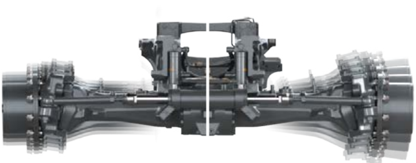
Front axle suspension The front axle suspension provides consistent suspension comfort no matter what the load or attachment, with position sensors controlling the level. This avoids any power hopping, increasing the tractive force on the front axle by up to 7% (compared to a front axle without suspension).
