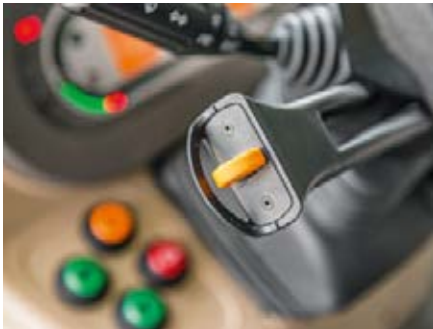
The button located steering wheel can be used to control reverse gear and the Stop & Go function.
