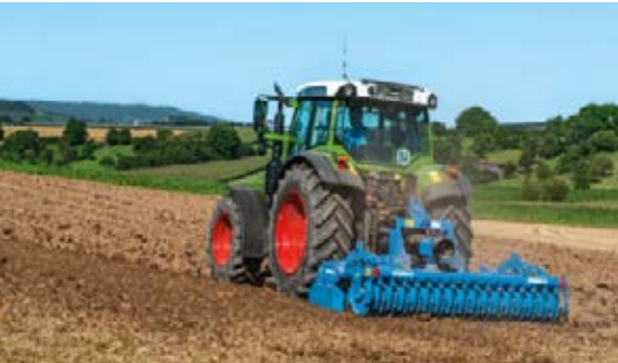
You can work with the correct PTO rpm at any speed thanks to independent control of road speed and engine speed.
