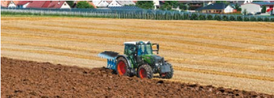
The TMS automatically controls the engine speed and gearbox ratio in the field for best efficiency with differing loads.
