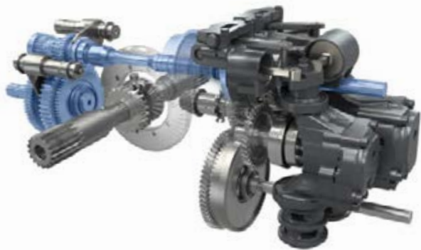
The Fendt Vario transmission ML75 is a continuously variable power split ground drive with one speed range. The hydrostats can be swung 45° and power-splitting via a planetary gear set ensures exceptional efficiency over the entire speed range.
