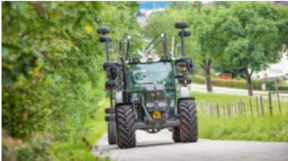
The tractor runs on level ground at a reduced speed. On a slope, the TMS increases engine speed and adjusts the gearbox ratio. As soon as the tractive power requirement is reduced, the TMS reduces the engine speed to the most fuel efficient range possible.
