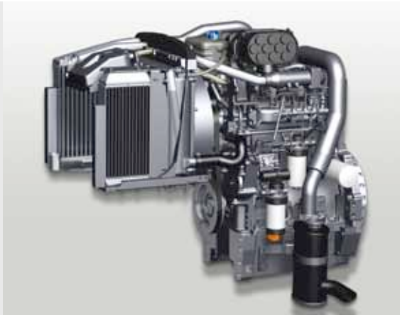
The 3-cylinder AGCO Power engine with external EGR technology The external EGR system provides targeted cooling of recirculated exhaust, which lowers fuel consumption considerably compared with internal exhaust gas recirculation systems. The latest technology in engine design has been implemented in the 3-cylinder AGCO Power engines, which allows the 200 Vario to attain high performance values while keeping fuel consumption low.
