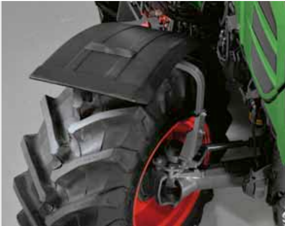
Pivoting mudguards The 200 Vario can be fitted with pivoting front mudguards as an option. They maximise the wheel angle and permit a turning circle of only 3.98 metres.
