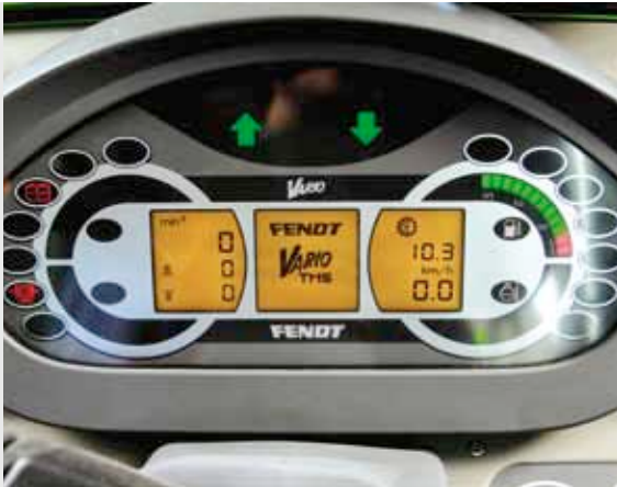
The clear multi-display The fuel consumption indicator on the 200 Vario is located in the multi-display. It provides information about the average and current fuel consumption and has two memories. You have full control at all times.
