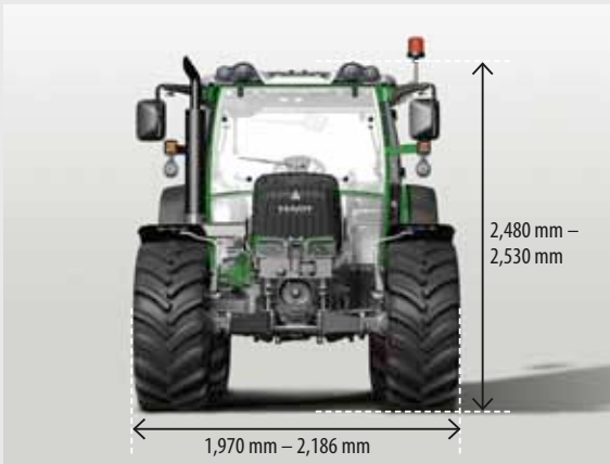
Low vehicle height for flexibility in the farmyard With a minimum vehicle height of 2,480 mm with 480/70R30 tyres, the compact 200 Vario is well-suited for driving into low storage buildings or stables.
