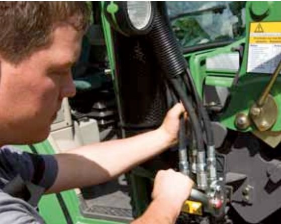
A multi-coupler connects all hydraulic and electric lines at once – even under pressure on the front loader side. The front loader can be quickly mounted and removed.
