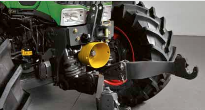
Interfaces at the front: • Top link • 7-pin socket • Front PTO • Lower link hook ends
