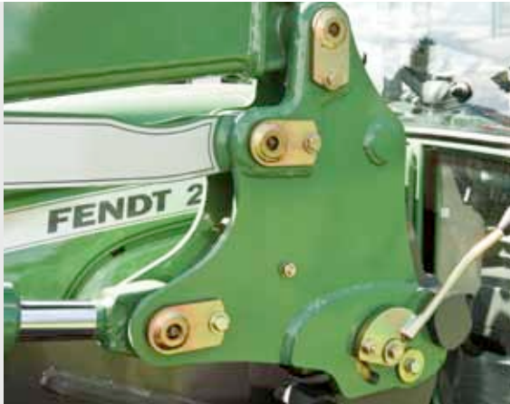
With the Fendt Cargo Lock, you can mount and remove the Cargo front loader from your 200 Vario even faster and easier. Thanks to the semi-automatic lock, you no longer need to insert locking bolts, which is often difficult. The system also offers optimum operational safety, since the front loader is locked in place immediately after driving into it.
