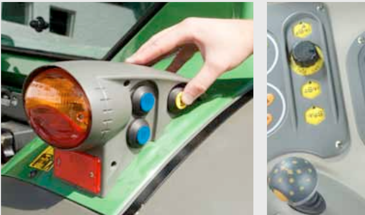
Save yourself unnecessary steps – ergonomic and convenient controls for the PTO The 200 Vario has external controls for the power lift and rear PTO. You can mount rear implements easily and save yourself unnecessary steps, for example, when filling the slurry tank.
