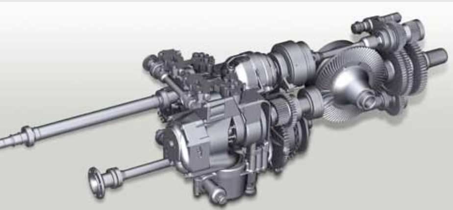
The ingenious Fendt Vario transmission The Fendt Vario transmission is a hydrostatic-mechanical power split drive. With increasing speed, the share of the mechanical power transmitted through the planetary set increases. The hydrostats can be swung 45 degrees and power-splitting via a planetary gear set ensures exceptional efficiency.
