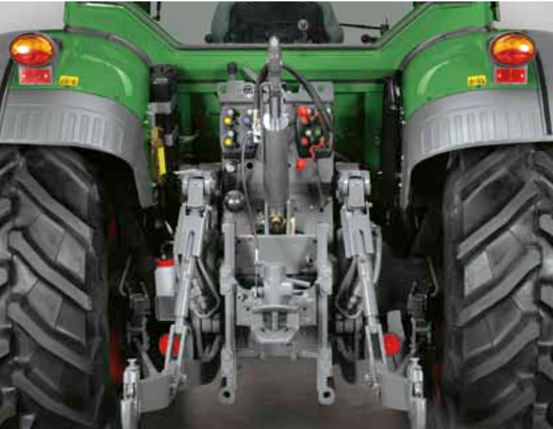
Clutter-free rear It is easy to find your way around at the rear of the tractor, because all connections are well designed and conveniently positioned.
