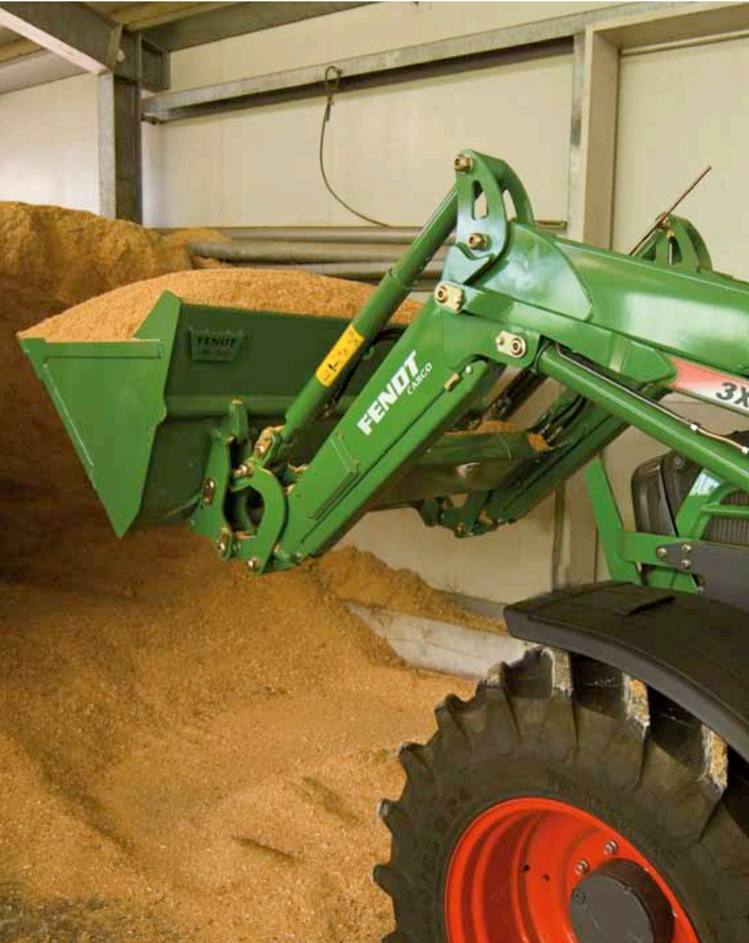
A multi-coupler connects all hydraulic and electric lines at once – even under pressure on the front loader side. The front loader can be quickly mounted and removed.
