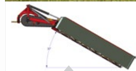
Side hitch attachment: makes mowing possible on sloping terrain
