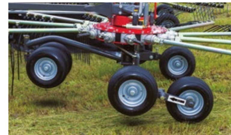
Patented, fully cardanic rotor suspension
