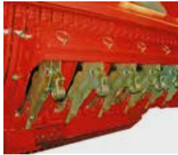
Bolt-on frame with 6 / 11 knives
