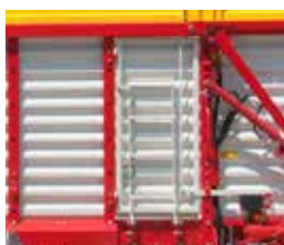
Access door with ladder
