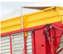
Roof ropes with rear tarpaulin
