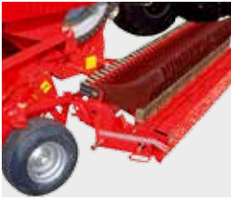
Knife bank swings out alongside wagon
