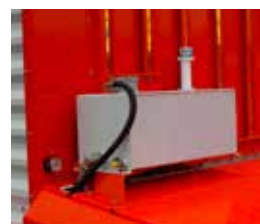
On-board hydraulics for cross conveyor belt
