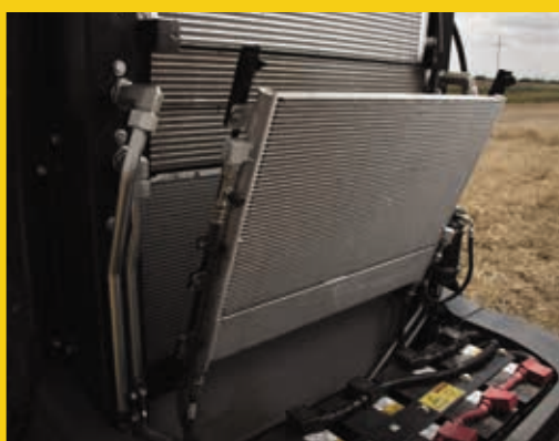
Engine cooling package with easy-to-clean two-plane design
