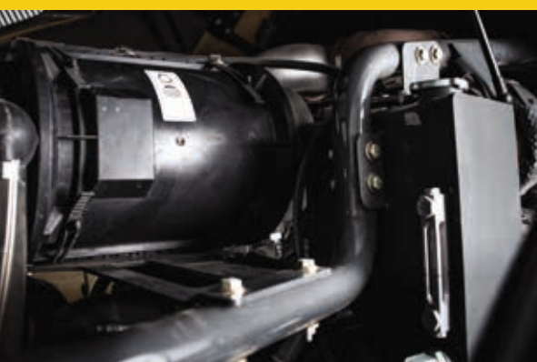
Engine air filter is easily removed and conveniently positioned
