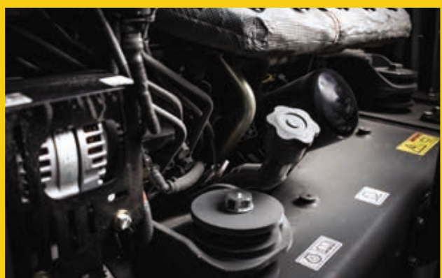
Engine oil can be checked and topped from ground level
