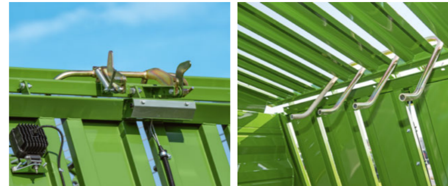
With the two-stage automatic loading system, light pressure is applied via a bar, while moderate pressure is applied via the loading flap.
