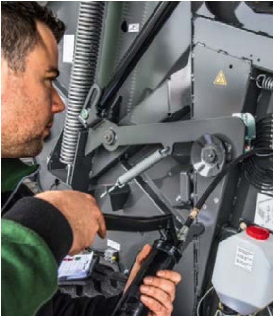
■ The lubrication points are consolidated here into one lubrication bar, making the system easy to lubricate.
