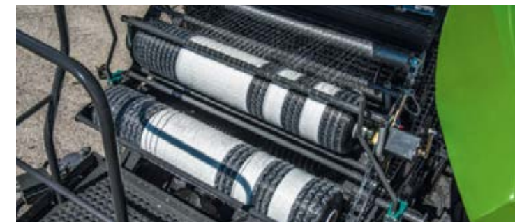
The EasyLoadSystem makes it possible to add net rollers in the shortest possible time.
