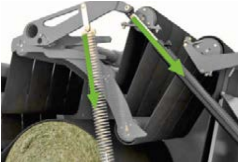
The small start chamber ensures a reliable and early core rotation. This forms the basis for perfect bales.
