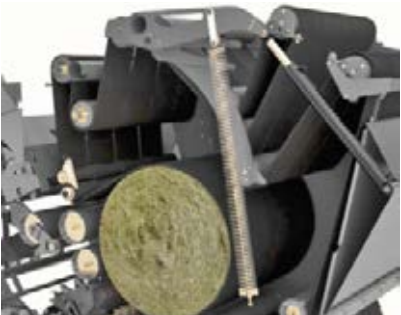
The two front belt-carrying rollers drive the belt. This double winding of the rollers means that the rotation is totally reliable for any type of bale.
