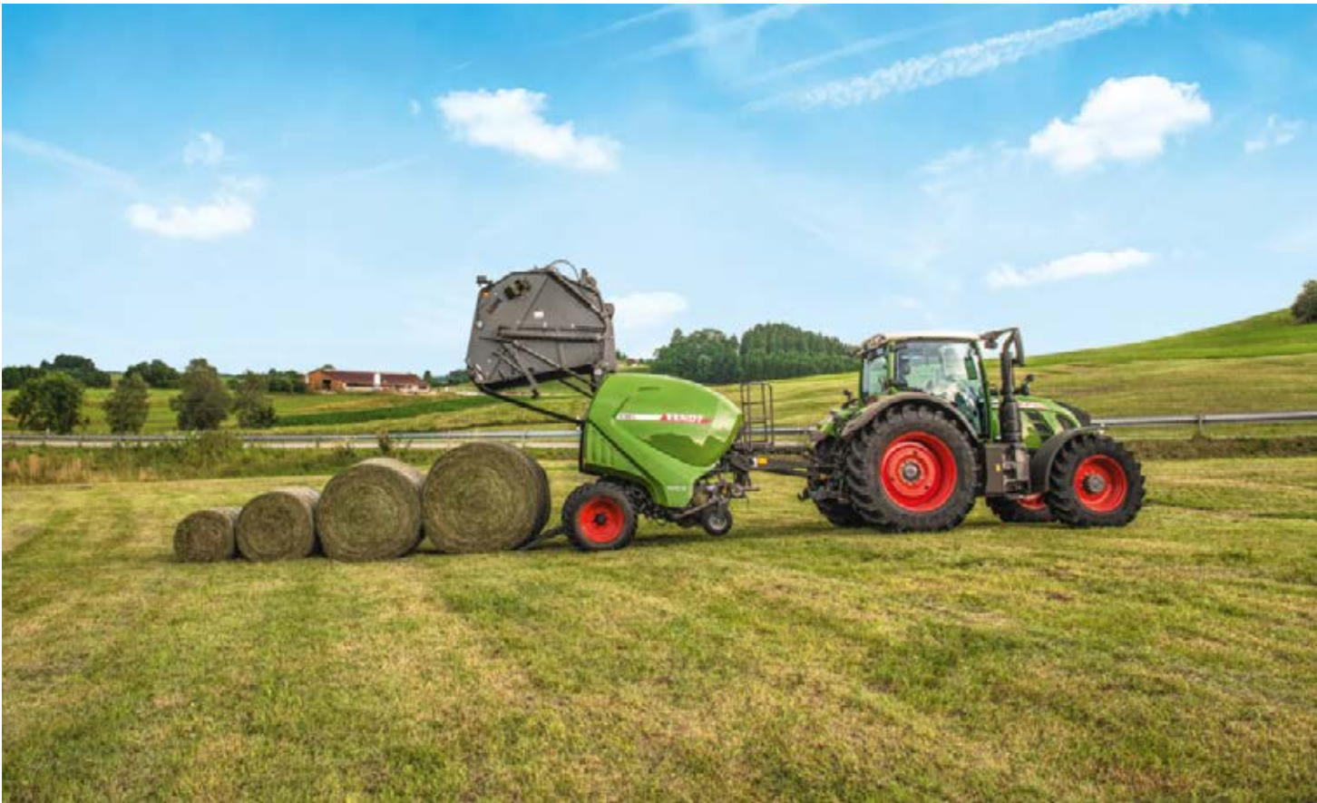
Variable Fendt round balers make it easy to compress bales with a diameter from 0.70 to 1.60 m or 1.80 m.
