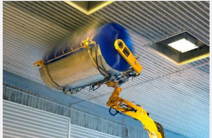
The tunnel washing brush TWB 2100 also cleans tunnel ceilings effectively.
