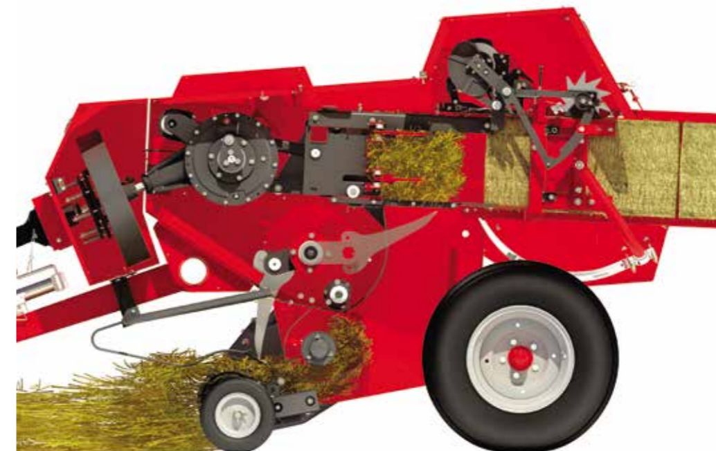
▲ The packer fork then pushes the pre-formed flake up and into the bale chamber.
