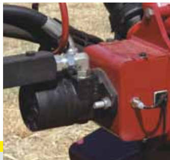
Hydraulic drive Ideal alternative to PTO shaft
