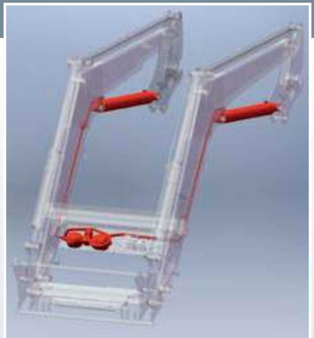
The two nitrogen tanks of the Manip'Activ suspension tared at different pressures.
