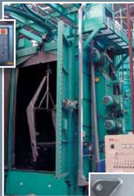
Shot-blasting of the loader parts and tools before painting
