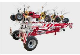
The trailed HIT T tedders with ten and twelve rotors are designed for really large areas. To meet the requirement of wider wide working width and still provide the best possible ground tracking, the rotor units are linked together by hinges. Combined with the chassis guiding the rotors, HIT T tedders guaranteed a perfect job even at higher working speeds.
