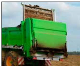
The Ferti-SPACE HORIZON muck spreaders is standard fitted, with a guillotine door. For further information, see page 12.
