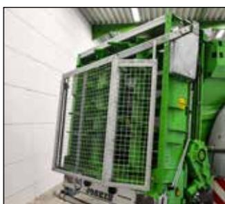
Protection grate for the beaters with hydraulic opening upwards (compulsory in some countries).
