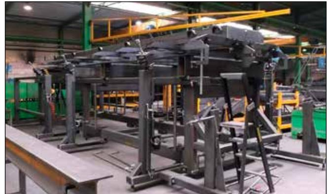
*The jigs used in the factory ensure precision and rapidity during the manufacturing process*
