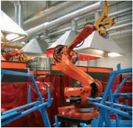
Robotised welding ensures accuracy and strength.
