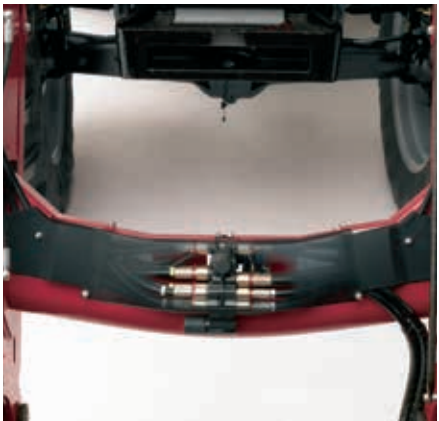
Cross-tube houses hydraulic components and provides strength.
