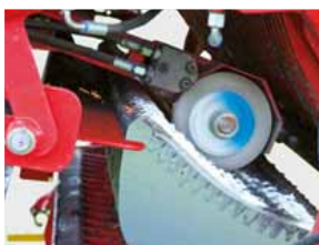
AUTOCUT On board knife sharpening
