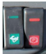
Three-speed transmission and park brake switches
